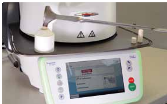
Place the cold IPS e.max Press Multi ingot into the hot investment ring, with the rounded, non-imprinted side facing forward. The imprinted side faces up to check the ingot shade.
