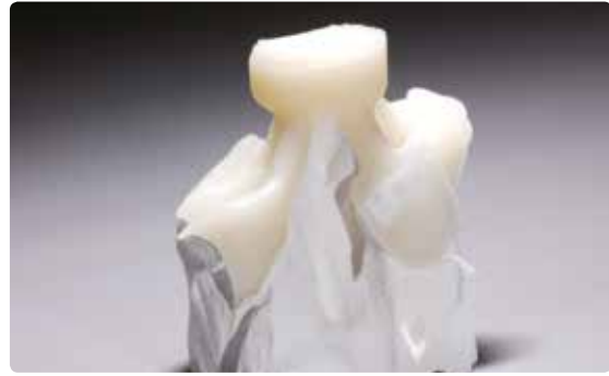
Fine divestment is carried out with polishing beads at 2 bar (29 psi) pressure.
