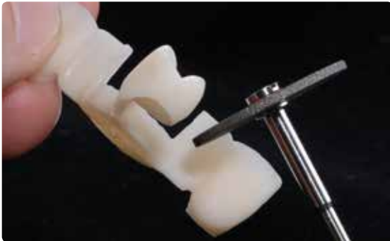
Separating the sprues in polychromatic restorations using a separating disc
