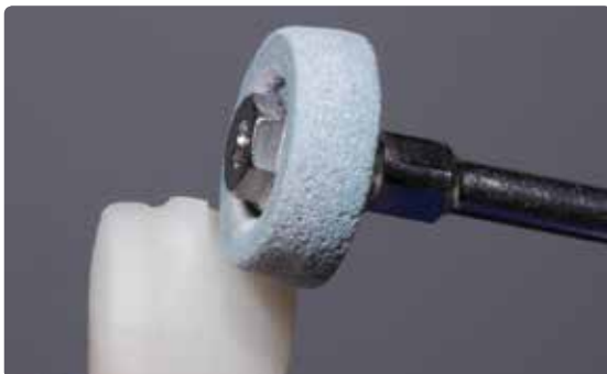
Smooth out the attachment points of the sprue using low speed and light pressure and finish the surfaces.
