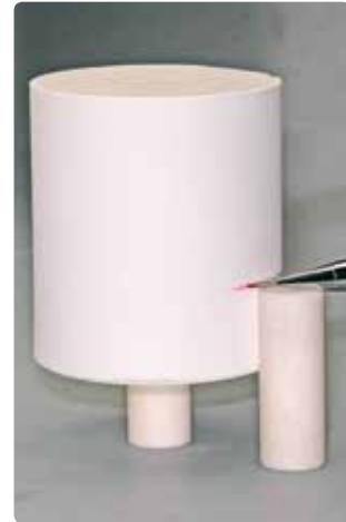
Mark the length of the Alox Plunger.
