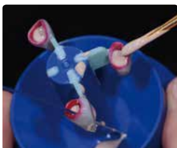
Carefully fill the cavities with investment material using a suitable instrument (e.g. brush).
