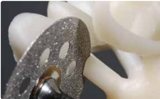
Separate the sprues with a thin diamond disc and provide permanent water cooling to the grinding area.
