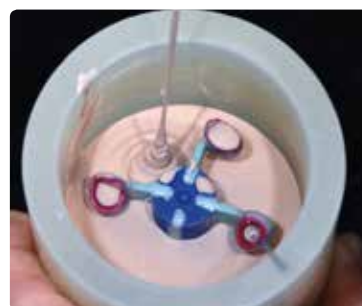
Pour the investment material slowly into the investment ring, so that the material can continuously fill the investment ring.
