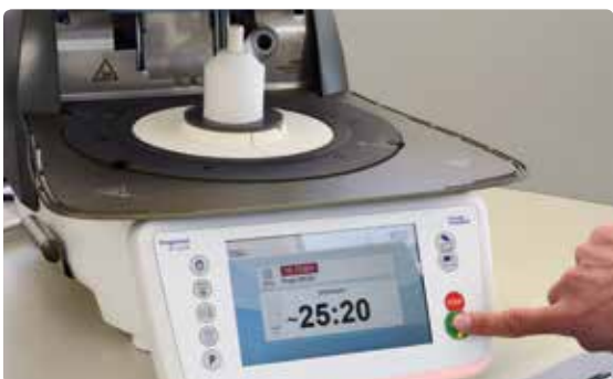
Place the loaded hot investment ring in the centre of the preheated press furnace using the investment ring tongs. Press START to start the IPS e.max Press Multi program.
