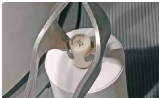
Place the cold IPS e.max Press ingot into the hot investment ring, with the shade imprint facing upward.
