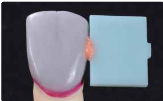
Sprueing may basically be performed from the mesial or distal. Apply a small drop of (soft) positioning wax on the side of the IPS Multi Wax Pattern. Press the restoration slightly against the soft wax.
