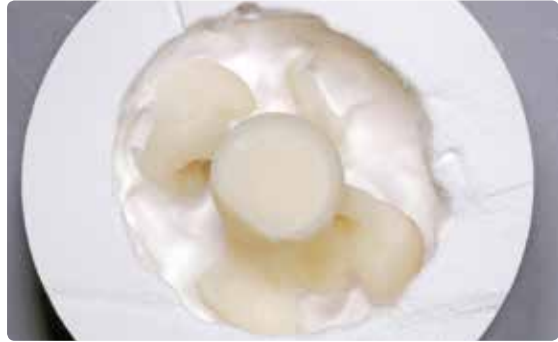
Rough divesting with polishing jet medium at 4 bar pressure until the objects become visible.
