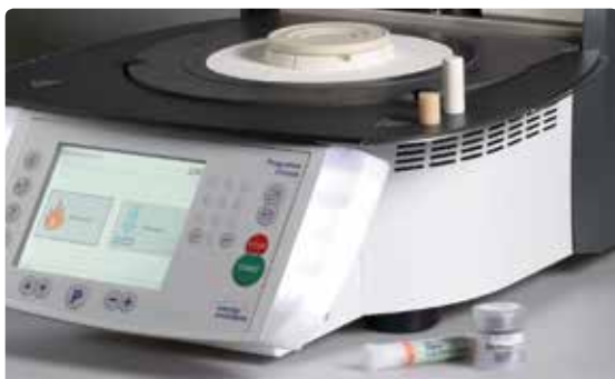
Provide a cold isolated IPS Alox Plunger and a cold IPS e.max Press ingot in the desired shade.
