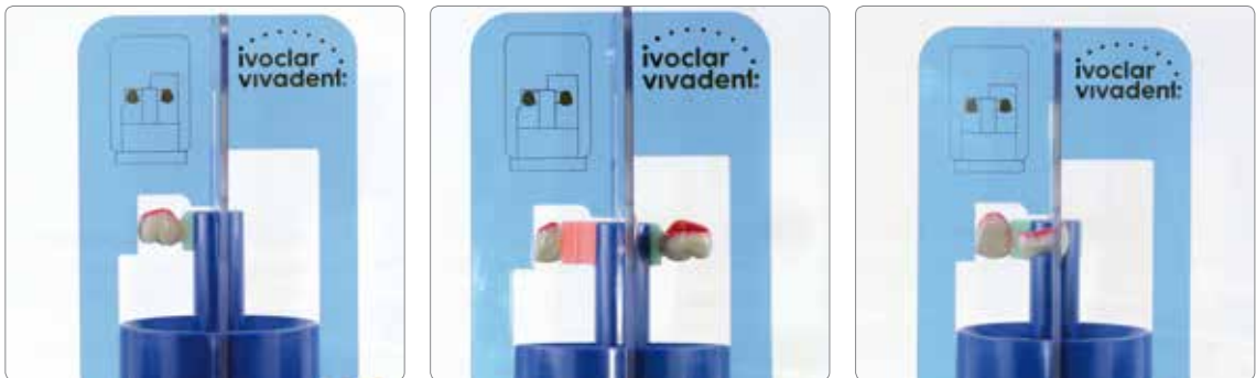
Attach the wax-up to the IPS Multi Investment Ring Base 200 g using the IPS Multi Wax Pattern. Check the correct positioning with the IPS Sprue Guide 200 g.
