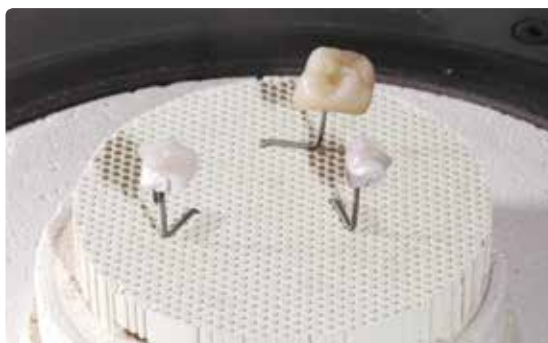
Conduct the Stain firing on a honey-comb firing tray belonging to the ceramic furnace.
