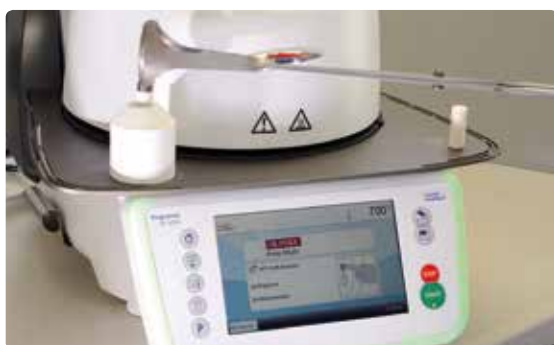
Place the cold IPS e.max Press Multi One-Way Plunger into the hot investment ring, with the rounded side facing forward.
