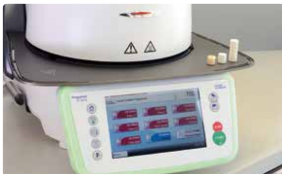
Provide a cold IPS Multi One-Way Plunger, a cold IPS AloX Plunger and a cold IPS e.max Press Multi ingot in the desired shade and select the press program for IPS e.max Press Multi.
