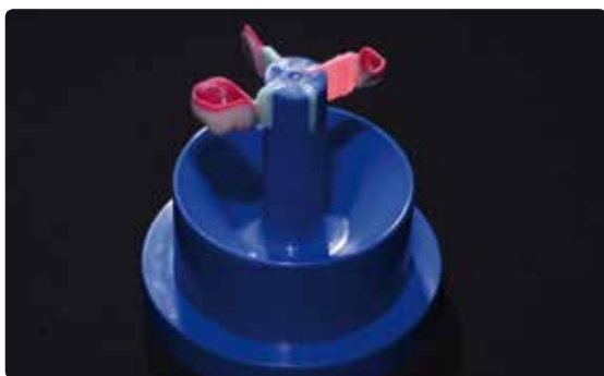
Prepared IPS Multi Investment Ring Base with wax-attached wax-up.
