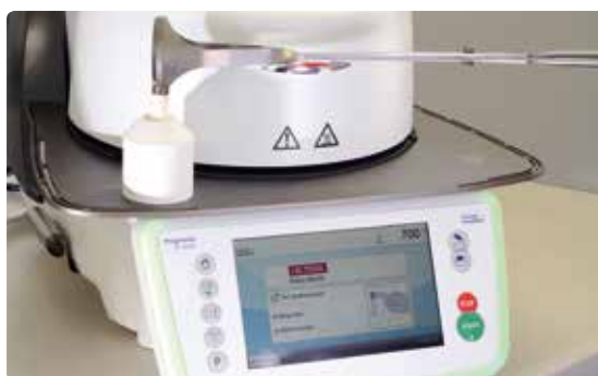
Place the cold IPS AloX Plunger in the hot investment ring.
