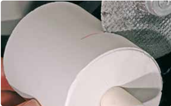
Separate the investment ring using a separating disc and break it at the predetermined breaking point.
